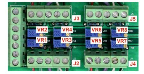
Adjustment of weighing cell J2 takes place at the potentiometer VR1 and VR2. Adjustment of weighing cell J3 takes place at the potentiometer VR3 and VR4. Adjustment of weighing cell J4 takes place at the potentiometer VR5 and VR6. Adjustment of weighing cell J5 takes place at the potentiometer VR7 and VR8. Increase the value turning to the right, reduce the value turning to the left.
