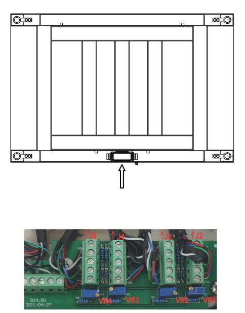
Adjustment of weighing cell J2 takes place at the potentiometer VR1. Adjustment of weighing cell J3 takes place at the potentiometer VR2. Adjustment of weighing cell J4 takes place at the potentiometer VR3. Adjustment of weighing cell J5 takes place at the potentiometer VR4. Increase the value turning to the right, reduce the value turning to the left.
