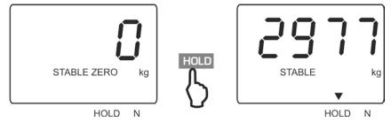
⇒ The peak load will be held on the display until deleted by pressing **HOLD**-key.
