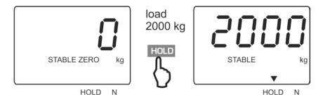
⇒ The weighing value will be held in the display until it is deleted by **HOLD**-key.
