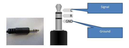
The FL-series have an analog output +/- 2V, the signal will be fetched directly at the load cell.
