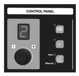
To regulate the level of aspiration to rotate the handle. The level of aspiration planned is suitable on the display.
